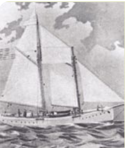
ILLUS 1. The artist's conception from Lewis & Dryden (1895). Note that the vessel is an "1890's" style rendering, with port lights (these would not have been available in Oregon country in 1840, and would have compromised the strength of a clinker-built hull) and the rig is wrong. Gale states: "... she had no topsails, but simply foresail, mainsail, gib and flying gib. Her spars were made of the straight fir sticks and consisted of... bowsprit and flying jibboom." The rig in this illustration has topsails, and neither flying jib nor jibboom. The U.S. Flag would have been properly carried on peak of the main gaff, not at the truck of the mainmast (Gale was a proper sailor!).
